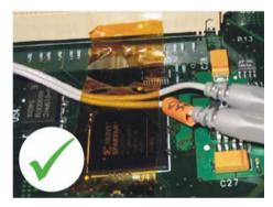
Figure 1-8 Correct securing methods
